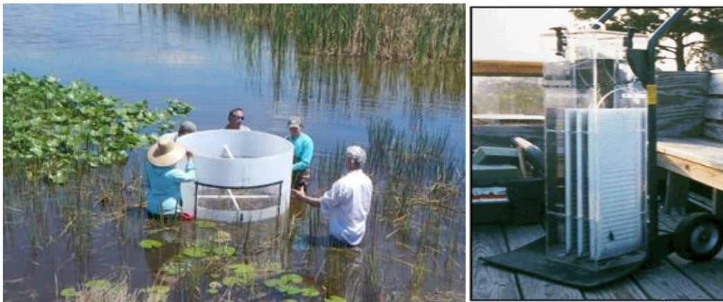
Figure 5C-5. P flux chamber in STA-2 Cell 1 (left) and porewater equilibrators (right) (photos by SFWMD).
