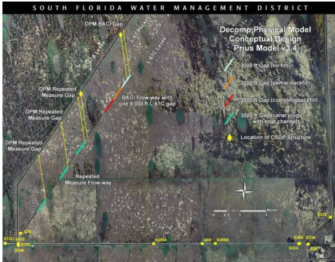
Figure 7. New hydrologic structures on the L-67A canals will move water out of WCA-3A and into WCA-3B as a controlled adaptive management experiment designed to look at the physics and ecology associated with sheetflow in a shallow peatland environment.
