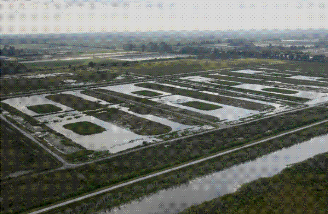
Figure 6. An oblique aerial view of the four, 15-acre macrocosm cells, with two 0.75-acre tree islands in each, soon after construction in 2001. Photo by SFWMD.
