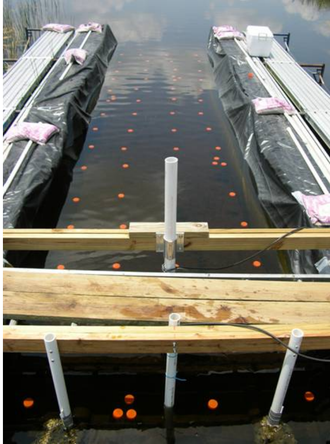
Figure 6-11. M1 flume at LILA used for tracer study. (Photo by SFWMD.) Orange caps indicate sampling locations. The Acoustic Doppler Velocity meter is located on the central PVC post. The tracer blocks (top of picture) were also added.
