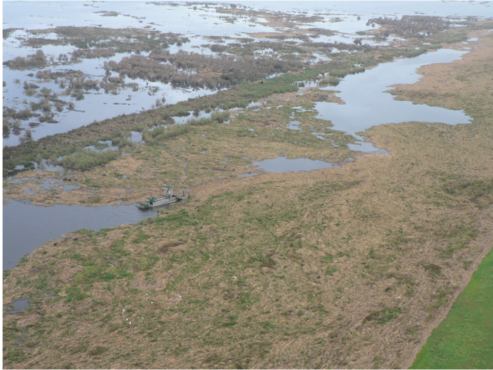
Figure 10-21. Dead vegetation in the Rim Canal being removed by an aquatic weed harvester (photo by SFWMD).
