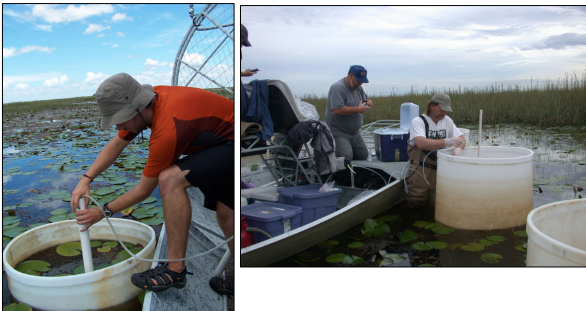
Figure 12. Soil (left) and interstitial water (right) sampling of mesocosms from an airboat. Airboats and operators were generously provided by the South Florida Water Management District (photo by Cynthia Gilmour, Smithsonian Environmental Research Center).
