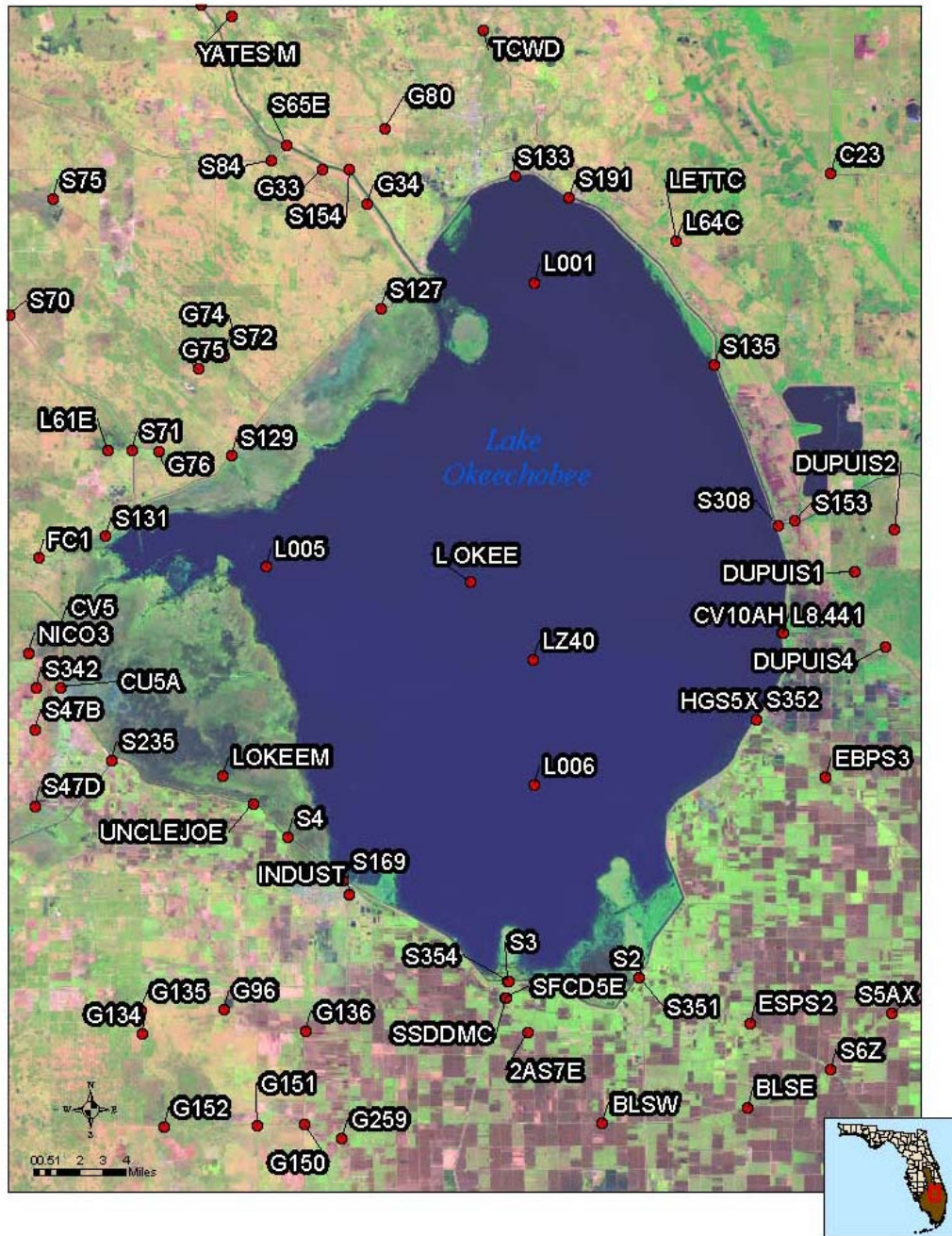
Figure 49. Water level recorders in Lake Okeechobee and the surrounding area.
