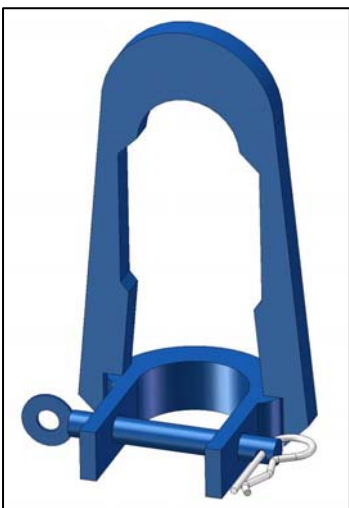
Wellpoint Puller – The wellpoint puller is fitted over the riser pipe and tightened against the pin, then lifted by the bail (either by hand or by machine depending on the depth) to pull the wellpoint from the ground.
