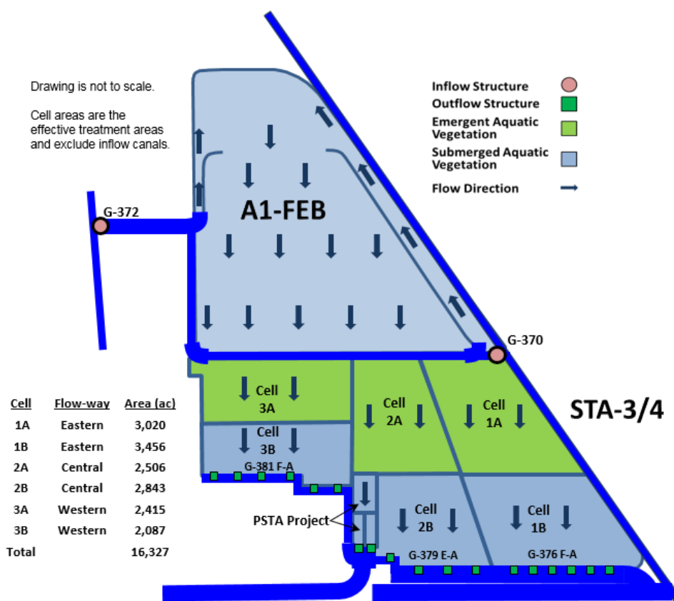
Figure 5B-10. Simplified schematic of STA-3/4 and the A-1 FEB showing major inflow and outflow water control structures, treatment area of each cell, flow direction, and dominant/target vegetation types. Treatment areas do not include pump stations, levees, roads, or other upland areas. Detailed structure maps of STA-3/4 and the A-1 FEB are provided in Appendix 5B-1 of this volume.
